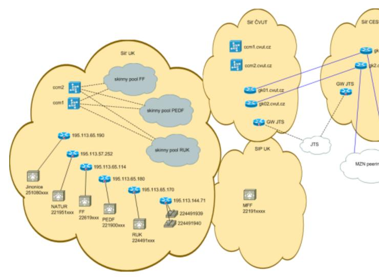
**Voice gateways** are usually routers equipped with the relevant interfaces (BRI, PRI) and instruments for digital processing of the signal (so-called DSP). Most frequently used are Integrated Services Routers (ISR) of platforms 26xx, 28xx, 38xx.
